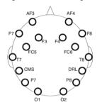
Figure 3. Electrode positions on the emotiv
